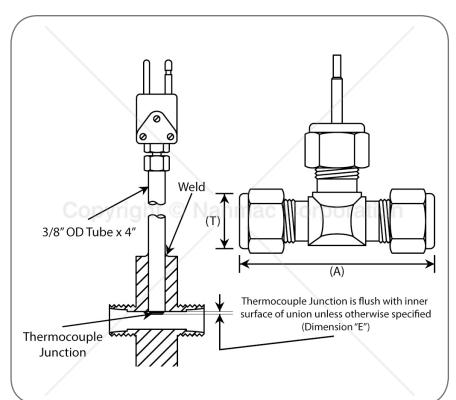
RTDs come standard with diaphragm. Thermocouples with a diaphragm are available upon request for sanitary applications
